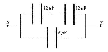
11. What is the equivalent capacitance of this combination of capacitors?
