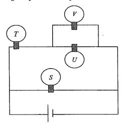
33. Bulbs S, T, U, and V all behave as identical ideal resistors in the circuit shown above. If bulb V is unscrewed, which of the following is true?
