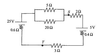
In the circuit above, the battery voltages and resistances are as indicated, with the internal resistances of each battery  $0.6~\Omega$  and  $0.4~\Omega$ , respectively.
